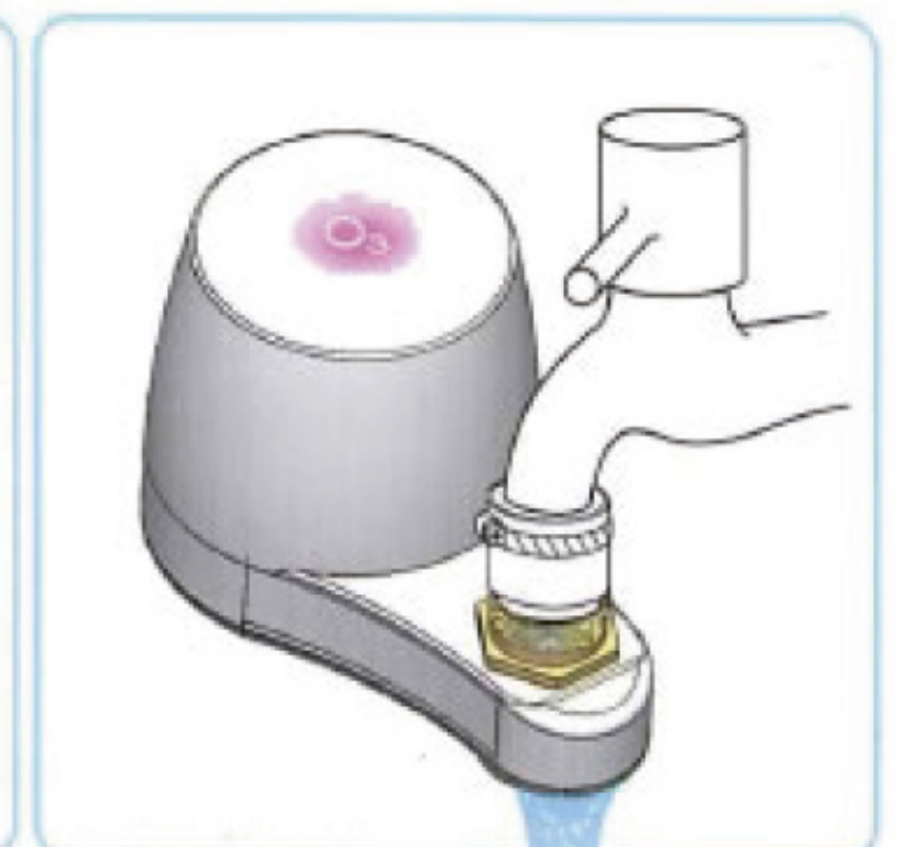
3. Open water check no leak then put transformer power on
